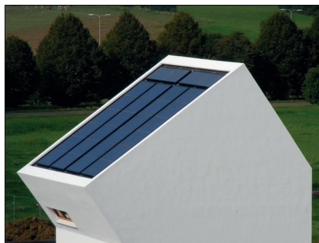
Figure 5. Photograph of the BIPV field test in 4 portrait BIPV segments and 2 landscape solar thermal collectors at the top.
